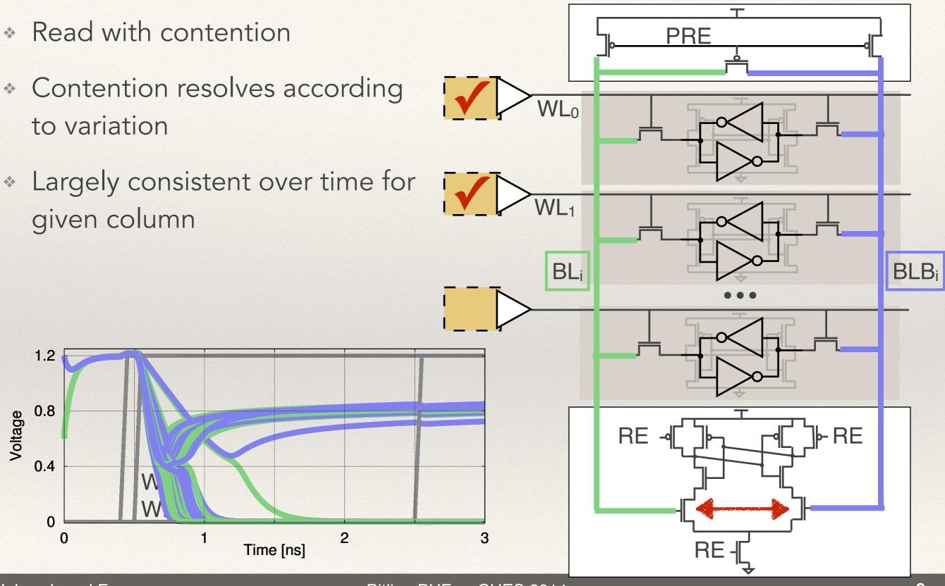
Read with contention PRE Contention resolves according \* WL<sub>0</sub> to variation Largely consistent over time for NL1 given column **BL**<sub>i</sub> **BLB**<sub>i</sub> Varies across columns or chips 1.2 0.8 Voltage - RE RE 0.4 M W 0 2 3 0 RE Time [ns]
