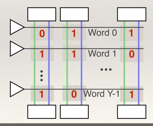
Adding a few gates to wordline drivers of SRAM creates a new PUF
