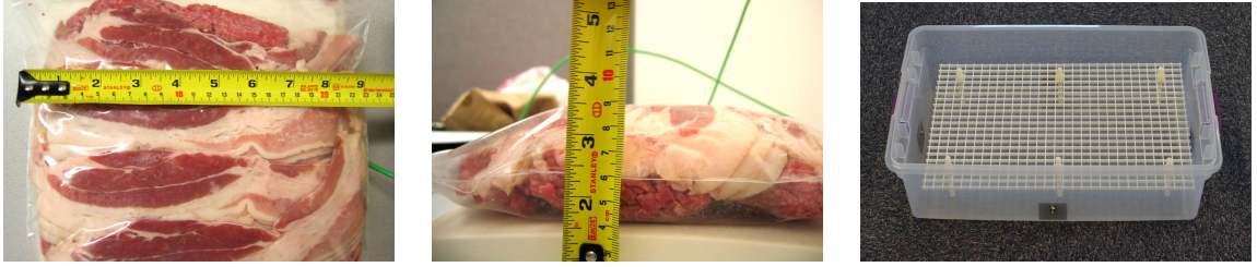
Figure 5.3. “Alice.” To simulate implantation in a human, we placed WISPer in a bag containing bacon and ground beef (left and middle). This method of tissue simulation is deprecated. Section 5.3.4 suggests a preferable method of tissue simulation (right).
