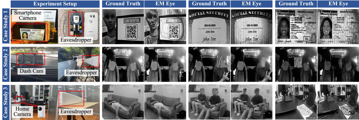
Figure 5.13: Three case studies of how EM Eye poses eavesdropping threats against smartphones, dash cams, and home security cameras. For each case, the experimental setup and three examples of ground truths and eavesdropped images are shown.
