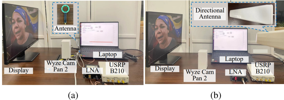
Figure 5.8: Experiment setups of using (a) a near-field probe within 10 cm and (b) a directional antenna beyond 10 cm.
